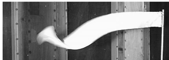
a) Photograph of loop A = 0.075 \text{ m}^2 , AR = 20 , U = 6.6 \text{ m/s} , and Re = 5.5 \times 10^5
